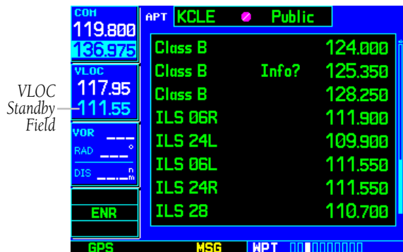
Figure 7-15 111.55 Moved to Standby Field
